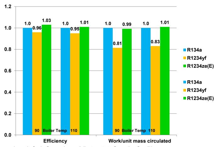
Thermodynamic Cycle Comparison - Adjustments to Operating Conditions
