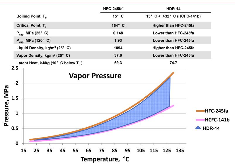
Replacement candidate has higher boiling point & T<sub>c</sub>
