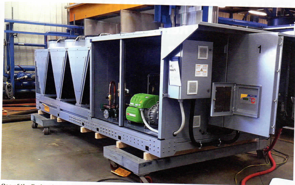
One of the Turbomiser chillers with its Turbocor compressor under test
