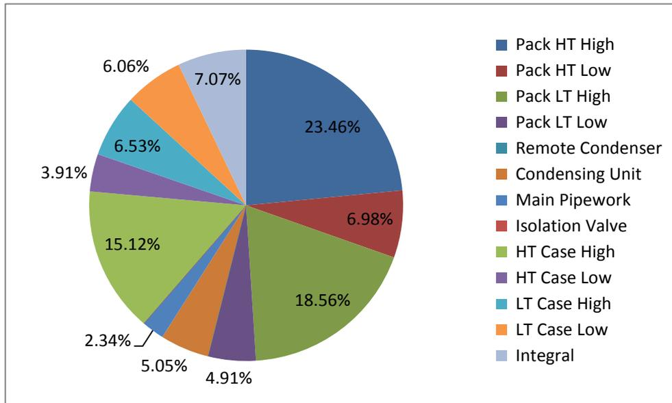
Figure 4 – 2011 Refrigerant leakage attribution.
