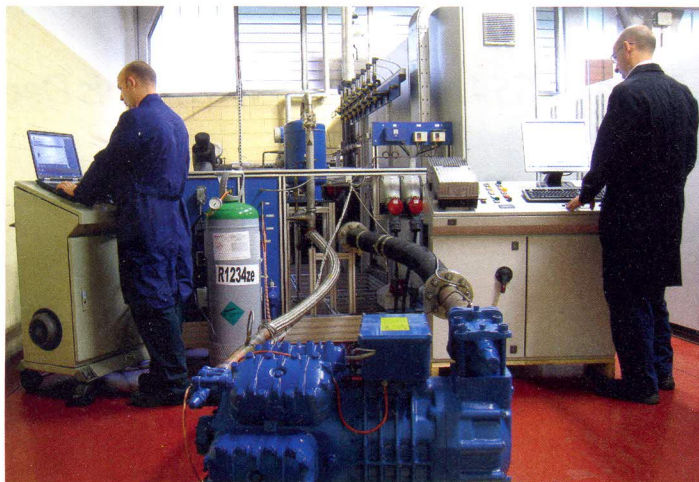
A Frascold 1234ze compressor under test
