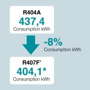
\* R407F' consumption is the estimated consumption that would have been provided with the refrigerant R407F under the same trial conditions for refrigerant R404A.
