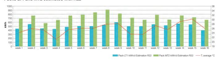
Comparison between Genetron® Performax™ LT and R22 in a LT and MT pack are shown below.
