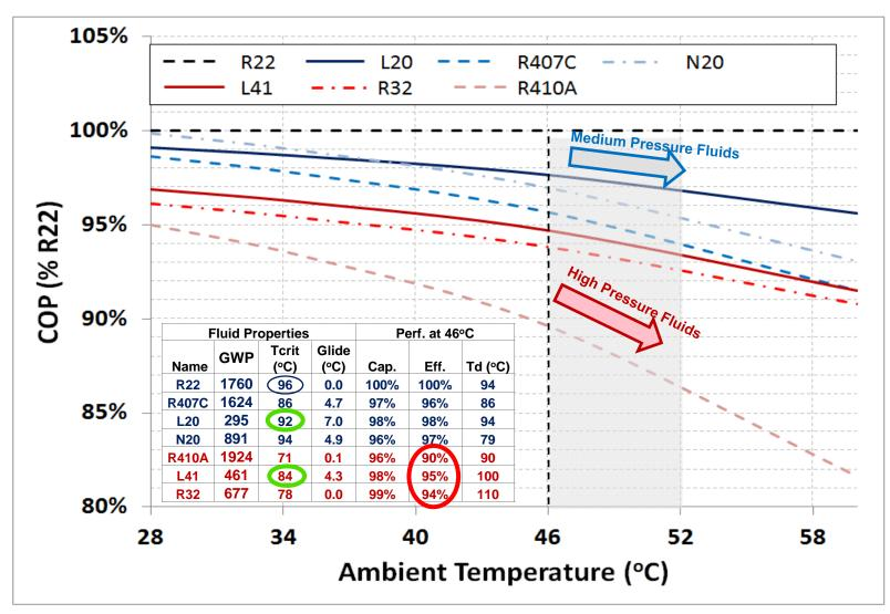
Condenser subcooling =  $5^{\circ}$ C; condenser TD =  $10^{\circ}$ C; Evaporating temperature =  $+10^{\circ}$ C; evaporator exit superheat =  $5^{\circ}$ C; suction line superheat =  $0^{\circ}$ C; volumetric efficiency = 100%; isentropic efficiency = 70%; Capacity equalized at  $35^{\circ}$ C ambient.
