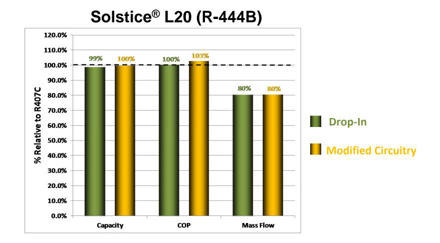
Drop In performance shows similar capacity (99%) and COP (100%) and lower mass flow (80%)
